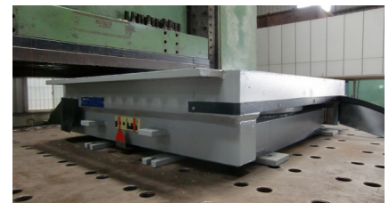
A RESTON®SPHERICAL bearing (guided sliding type) before installation to support a box girder
