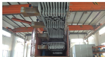
A TENSA®MODULAR expansion joint, made in mageba's production facilities, during loading
