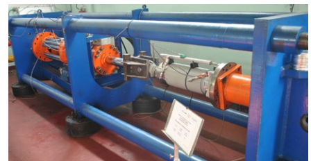
All 296 RESTON®SA dampers were successfully tested before installation
