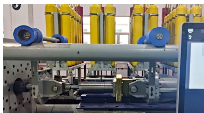
Testing of a RESTON®SA damper in Shanghai
