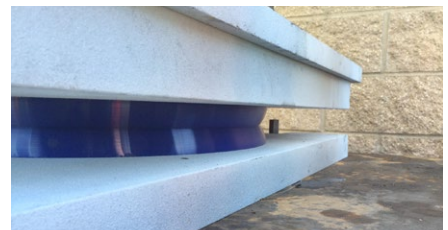
RESTON®DISC bearing during load testing
