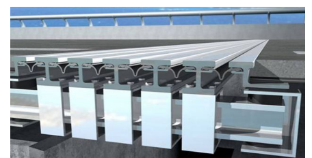
Deck movements will be facilitated by modular joints (as shown) and sliding finger joints
