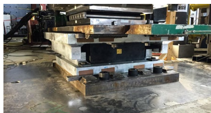
The bearing after 72 hours of cooling at -30 °C
