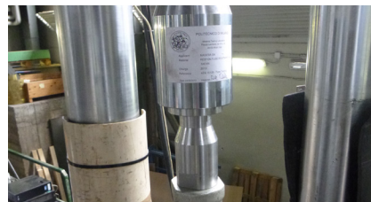
A fuse element (without shock absorber) in testing at Politecnico di Milano, Italy
