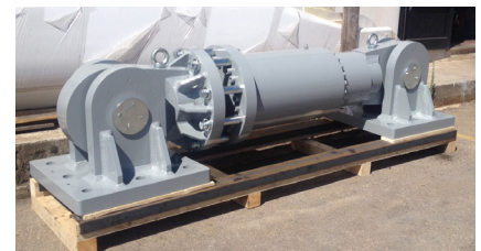
A shock absorber, fully assembled with fuse element and ready for transport to site
