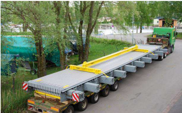
Figure 5. The Chongming Bridge over the Yangtse River near Shanghai (left), and one of its 22-gap Tensa-Modular joints during transport to site (right)
