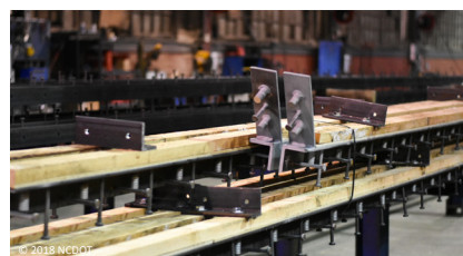
TENSA®FORCE joints during assembly in the factory
