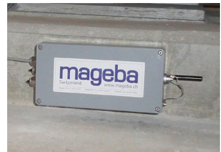
Data acquisition unit of a monitoring system
