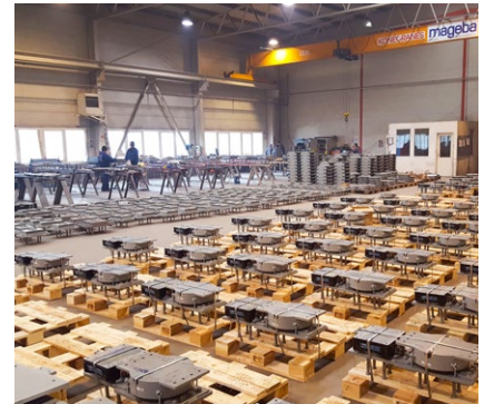
mageba in house production facility of structural bearings
