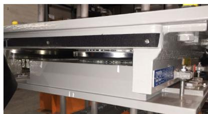
Installed RESTON®SPHERICAL bearing
