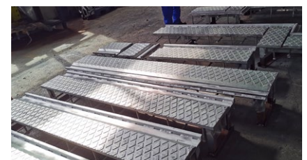
Joints after assembly in mageba's Shanghai facility
