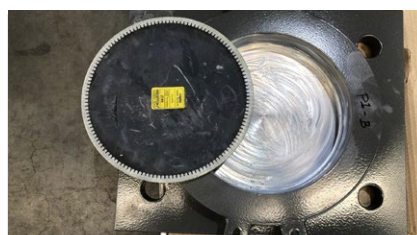
A RESTON®POT HP bearing during manufacturing
