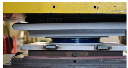
One of the project's RESTON®DISC bearing being load tested per AASHTO LRFD, after fabrication
