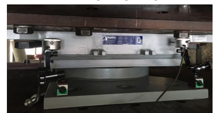
A RESTON®POT bearing during testing
