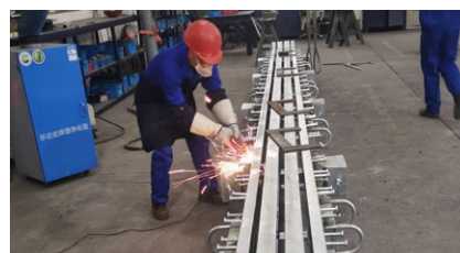
One of the modular joints during assembly in mageba's Chinese production facility
