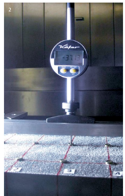
1 Over-rolling test using truck tyres 2 Movement capacity test on a TENSA®POLYFLEX®RapidCure specimen of type RC60
