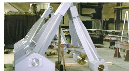
Two wind shoes, ready for delivery from the factory in Switzerland
