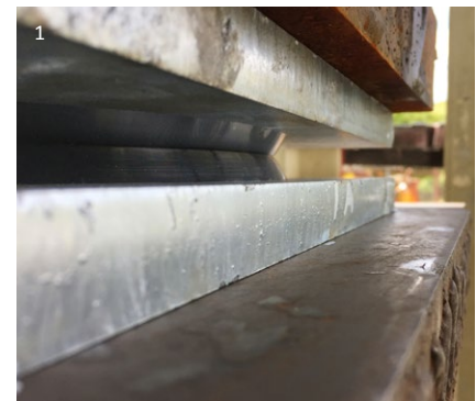
1 Testing of a disc bearing to 150 % proof load, per AASHTO LRFD specifications.
