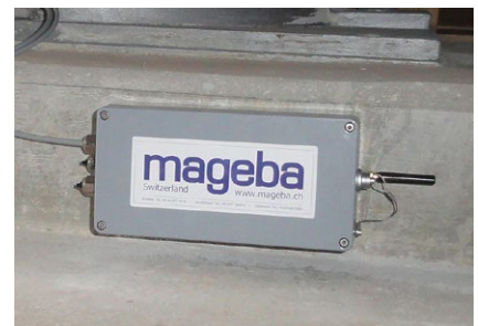
Data acquisition unit of a SHM system
