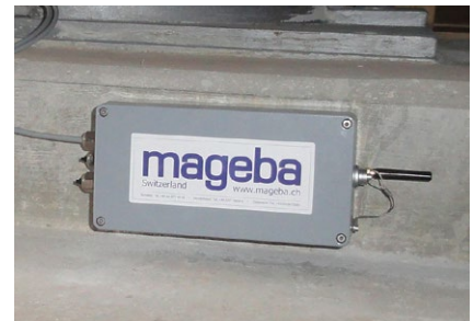
Data acquisition unit of a SHM system
