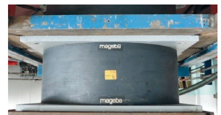
Full-Scale Sample LASTO®LRB prepared to be tested under actual seismic conditions in Italy
