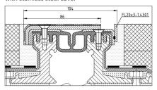
Installed joint with non-skid cover plate
