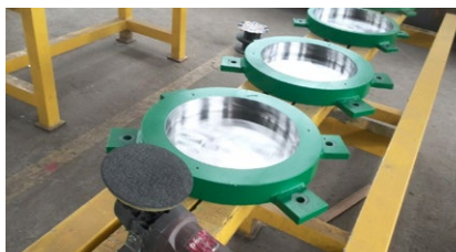
mageba RESTON®POT bearings during production
