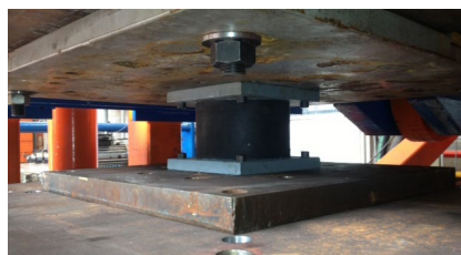
Testing of a LASTO®LRB lead rubber bearing prior to installation
