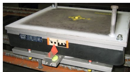
A RESTON®POT bearing of type TE after production
