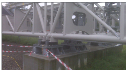
Rigorous testing of the APM system, including bearings, was carried out on a special test track.
