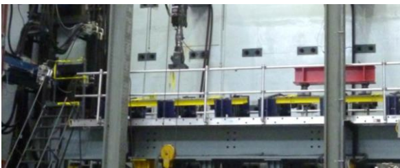
Figure 6. Fatigue testing of the specific type and design of modular joint – testing rig at ATLSS / Lehigh University
