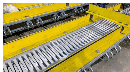
Assembly of finger joints in the factory
