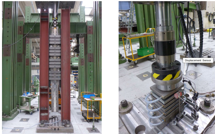
Fig. 2) a) Wear test setup and b) fatigue test setup both with active temperature control
