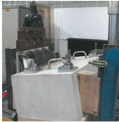
Fig. 5) Fatigue testing of anchorage
