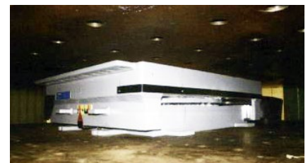
Spherical bearing being tested according to AASHTO
