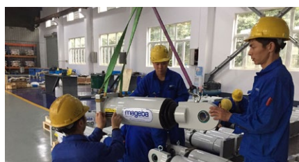
Labelling of viscous dampers at mageba's Shanghai factory following fabrication
