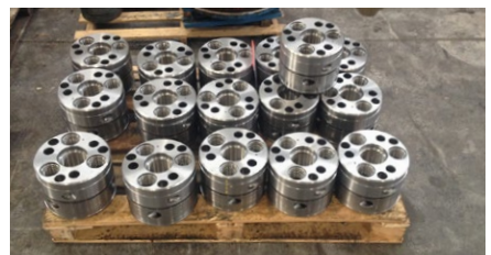
Parts of the RESTON®SA shock absorbers as fabricated, prior to assembly of the dampers
