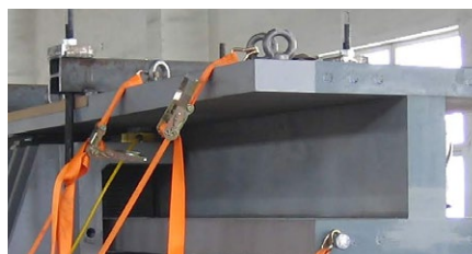
Preparing the special bearings for transport
