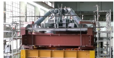
Testing of one set of four RESTON®SA shock absorbers, arranged as used in roof canopy
