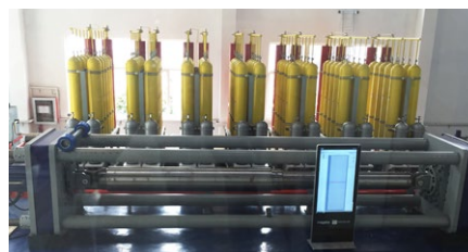
Testing of a RESTON®SA shock absorber in Simalab, Shanghai
