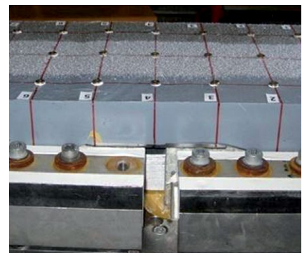
Movement capacity tests Tensa®POLYFLEX® Advanced PU
