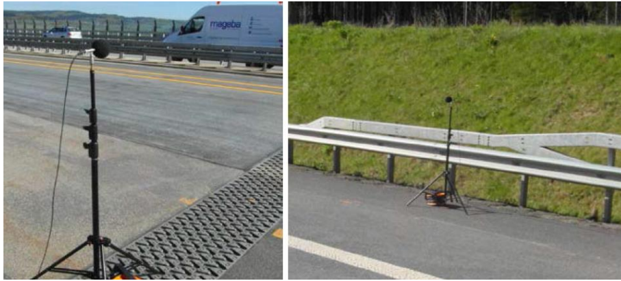
Figure 7. Measurement of noise at a 5-gap Tensa-Modular joint on the Liesertal Bridge on the A1 auto-bahn in Germany – directly at the expansion joint (left), and at a distance of 30 m away (right).
