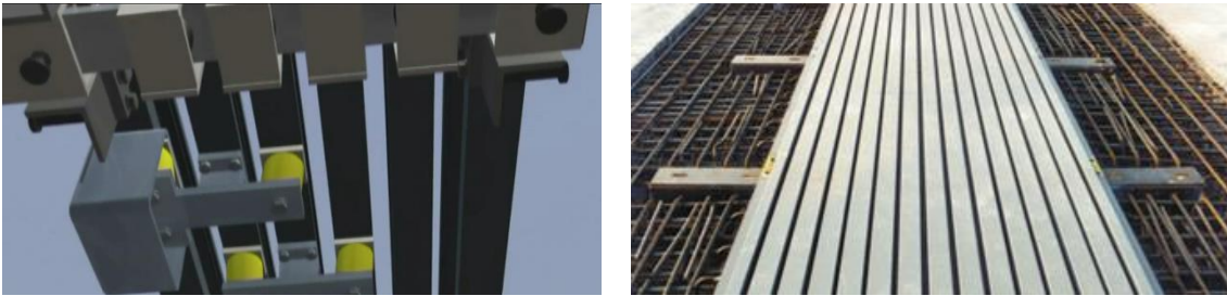
Fig. 5. The design of the modular joint type shown in Figure 1 helps combat noise; its elastic design (left) provides damping and prevents impacts between its structural elements, and its regular, rectilinear layout simplifies installation, minimizing the risk of noise due to sub-optimal installation.
