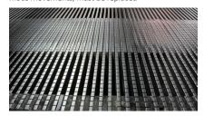
3D view of a new sliding finger joint, facilitating longitudinal movements of 2,700 mm
