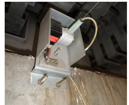
Ultrasonic sensors installed on the joint
