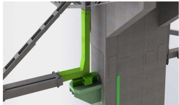
Figure 2. Illustration showing developed solution (highlighted) with part of deck truss replaced and supported by a new bearing on a new support bracket which projects out from the tower
