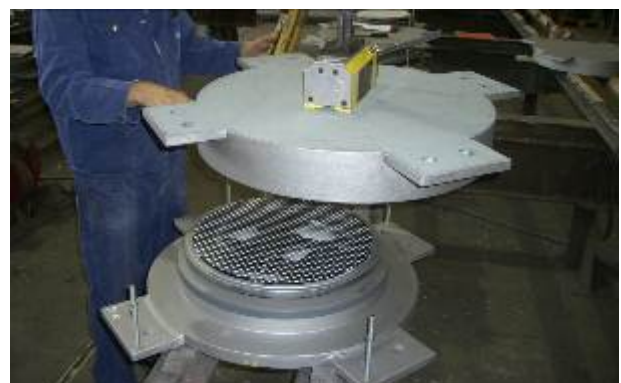
Figure 6. Assembly of a fixed spherical bearing
