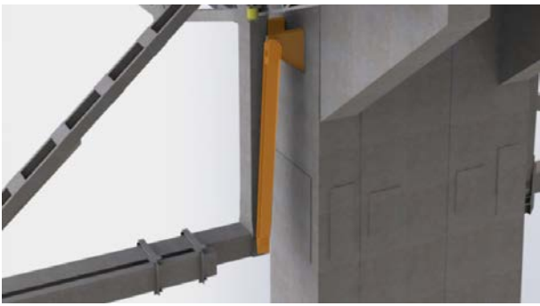
Figure 1. Illustration showing a Truss End Link (highlighted) at end of one section of deck truss. Pins at both ends allow the link element to rotate, enabling deck movements to be accommodated
