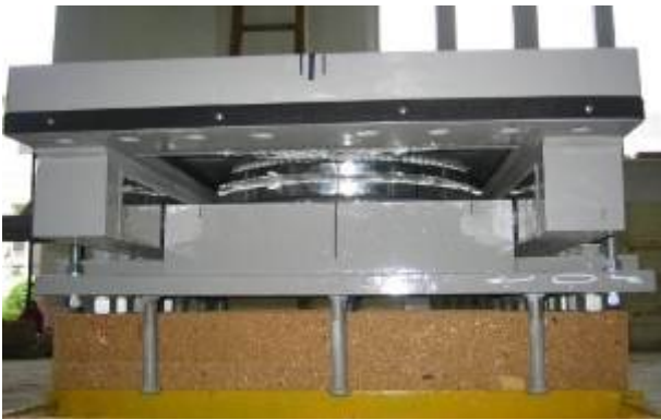
Figure 7. A guided sliding spherical bearing
