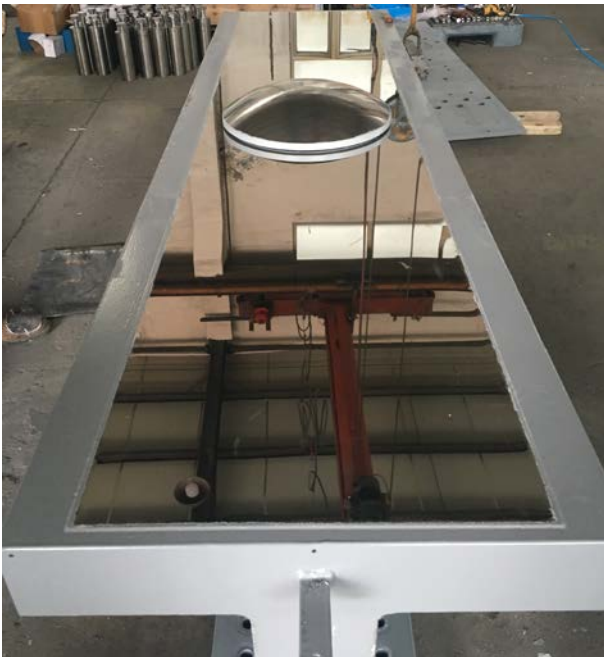
Figure 14. View of top of longitudinal T-beam, with stainless steel sliding sheet applied to top surface and calotte of spherical bearing positioned on top
