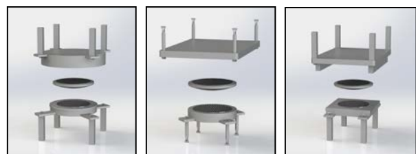
Figure 5. Exploded views of spherical bearing types (from left: fixed, free sliding and guided sliding)
