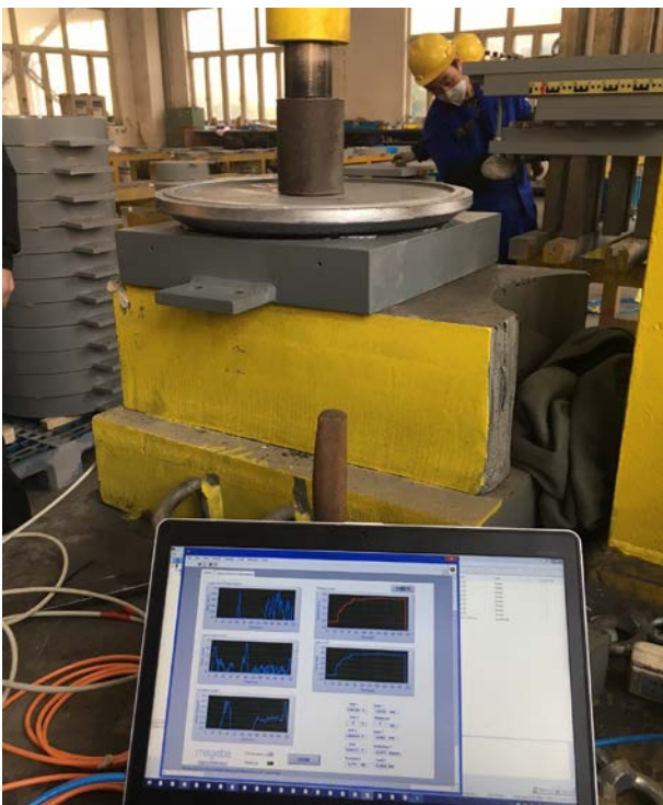
Figure 18. Testing of a piezoresistive pressure sensor following integration in a bearing
