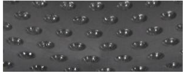
Figure 8. Close-up view of Robo-Slide (with grease dimples) – a high grade alternative to PTFE for bearings and expansion joints
