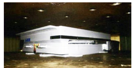
Spherical bearing being tested according to AASHTO
