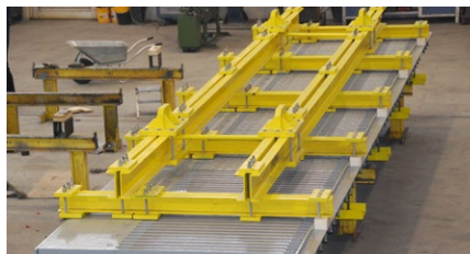
Sliding finger joint with transportation and installation frame, ready for delivery
