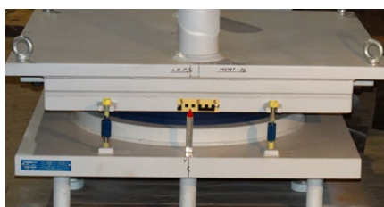
A finished Disc bearing before delivery
