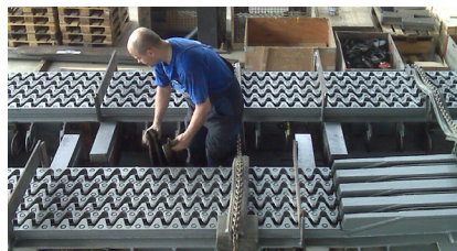
Securing of two TENSA®MODULAR expansion joints with sinus plates on a truck for transport
