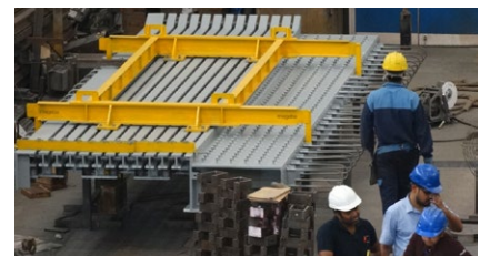
The modular joints were fabricated at mageba's Indian factory in Kolkata
