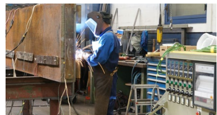
Bearing production in Switzerland: the massive sliding plates feature 5.5 t weight and 3.2 m
