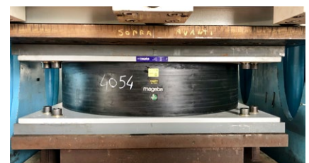
LASTO®LRB under laboratory testing
