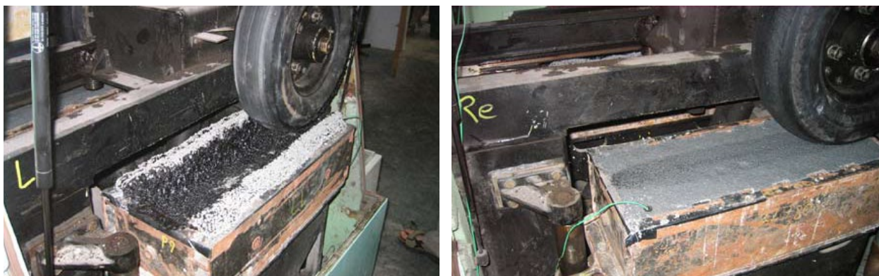
Figure 11: Comparison of flexible plug materials after rutting test per EN 12697-22 at 60°C. (Left: Common asphalt plug after 100 cycles. Right: PU material of described joint after 30,000 cycles)
