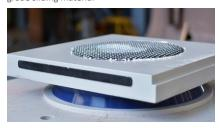
One of the project's RESTON®DISC bearing being load tested per AASHTO LRFD, after fabrication
