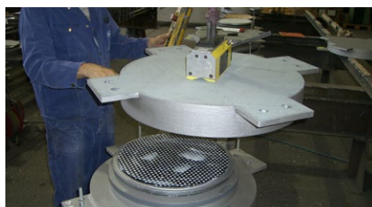
Assembly of a RESTON®SPHERICAL bearing, showing its upper greased ROBO®SLIDE disc
