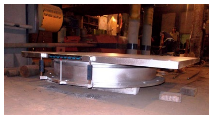
A RESTON®POT bearing with capacity of 18,000 kN as fabricated and ready for delivery to site.
