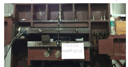
Load testing of the RESTON®SPHERICAL bearings
