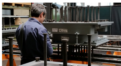
Fabrication of a RESTON®POT bearing in mageba production hall
