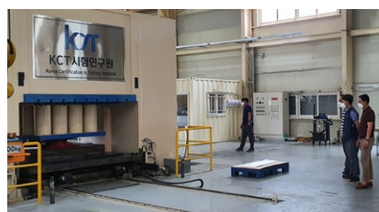
Testing of a standard RESTON®PENDULUM isolator bearing
