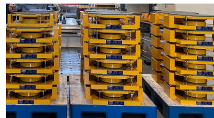
RESTON®PENDULUM bearings are ready to be tested
