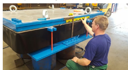
Assembly of a bearing in the workshop
