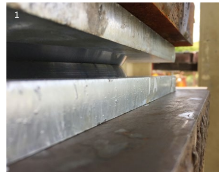
1 Testing of a disc bearing to 150 % proof load, per AASHTO LRFD specifications.
